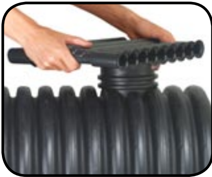
This Corru-Tap is one way to connect to the transport system in a horizontal application. It connects 12-inch Multi-Flow to a corrugated pipe. A similar connector is available for 6-inch Multi-Flow. Rigi-Taps are used for connections to PVC pipe.
